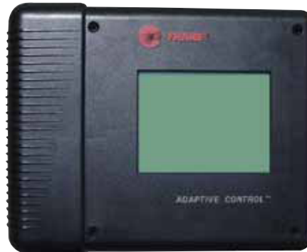
Fig. 23 – DynaView operator interface
